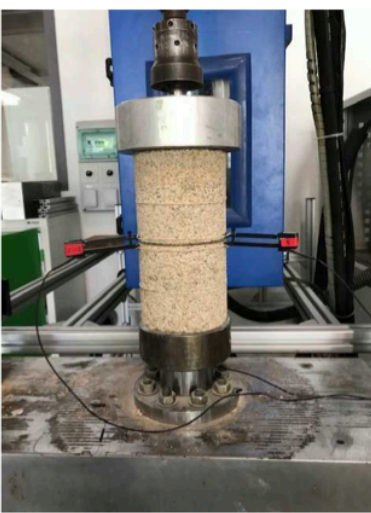
Mechanical test (compression, Bending) of Rice Husk Concrete
