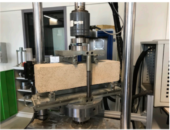
Mechanical test (compression, Bending) of Rice Husk Concrete
